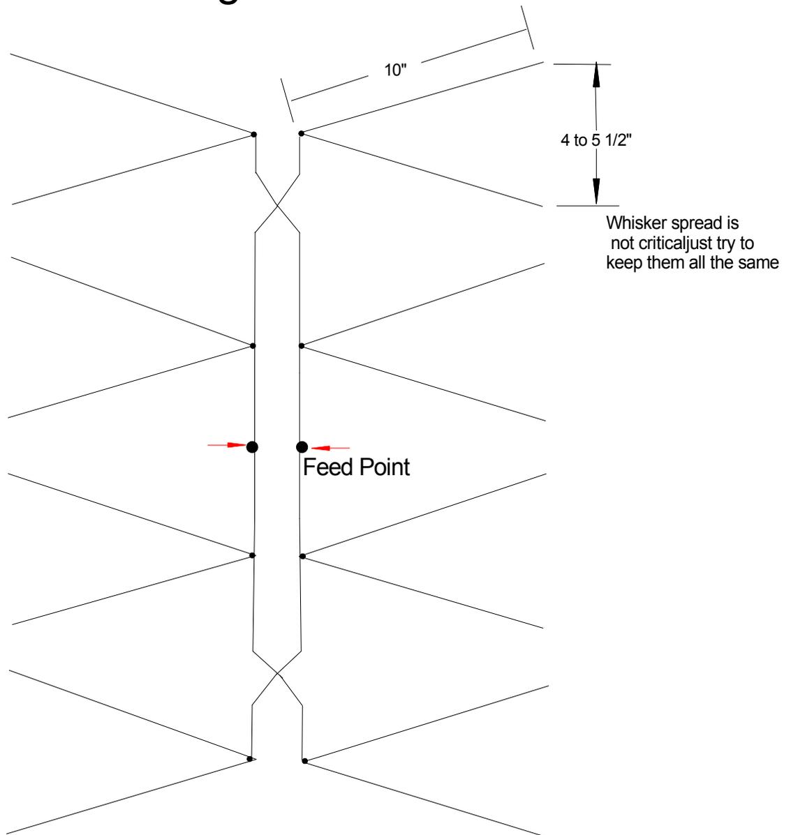
Most any metal will work for the elements. Try to use something near 1/8" diameter and make sure they are free of all coatings and oxidation where they connect to the phase line.
